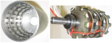
Fig. 2. Prototype of a TFM, (left) rotor, (right) 3 stack stator
